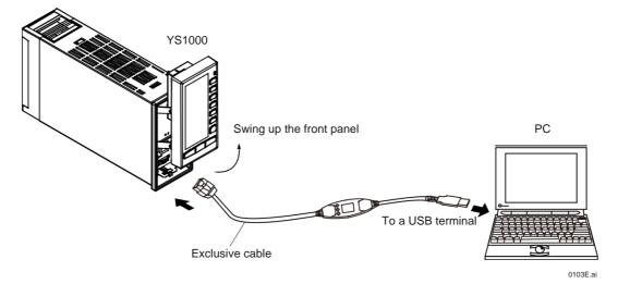
Note: The communication port inside the front panel of the YS1000 is incorporated into the YS1000 as standard.
