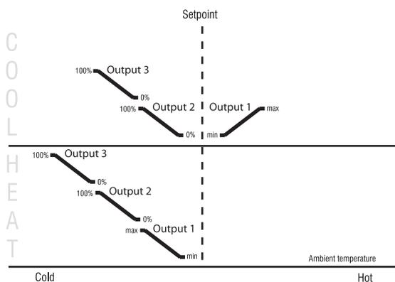
When setting 5 is selected, Output 3 controls heating or cooling depending on whether the default mode has been set to heat or cool respectively (see section 4.3.1). For example, if the default mode has been set to heat mode, the contact remains opened when the thermostat is in cool mode. When the thermostat is in heat mode, the contact closes when Output 1 reaches a percentage of its capacity, set via the configuration menu.
