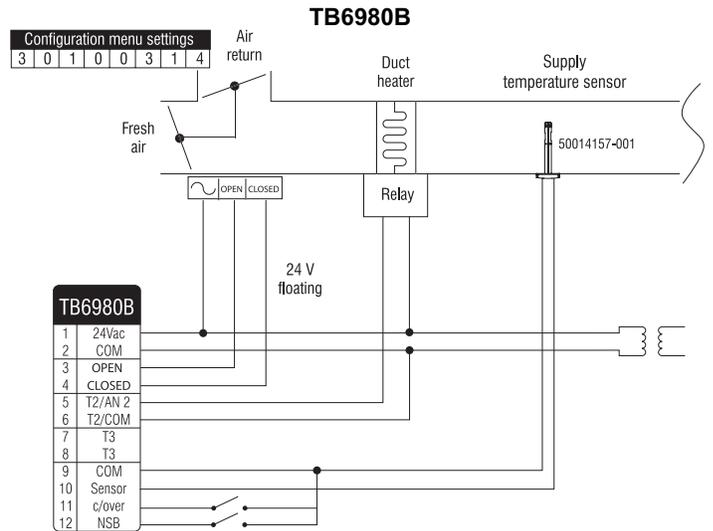
**FIGURE 4:** Temperature control of fresh air supply
