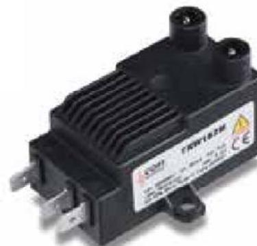
Ignition transformer with capacitive discharge technology for applications in condensing boilers and atmospheric gas burners. Developed to produce more power to the classics on board lighters, filtered against electromagnetic interference and available with output for mono-electrode flame detection.
